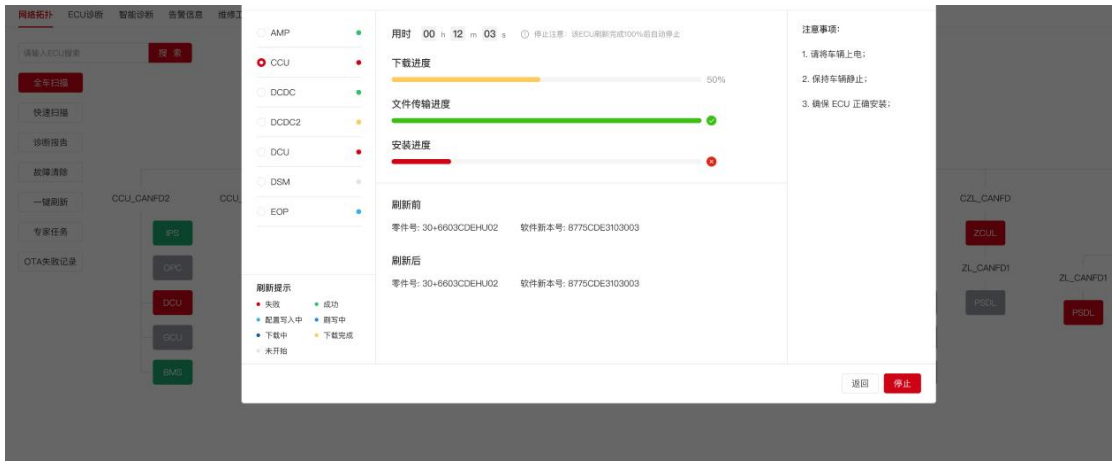
Figure 4-26 Parallel Flashing in Progress
